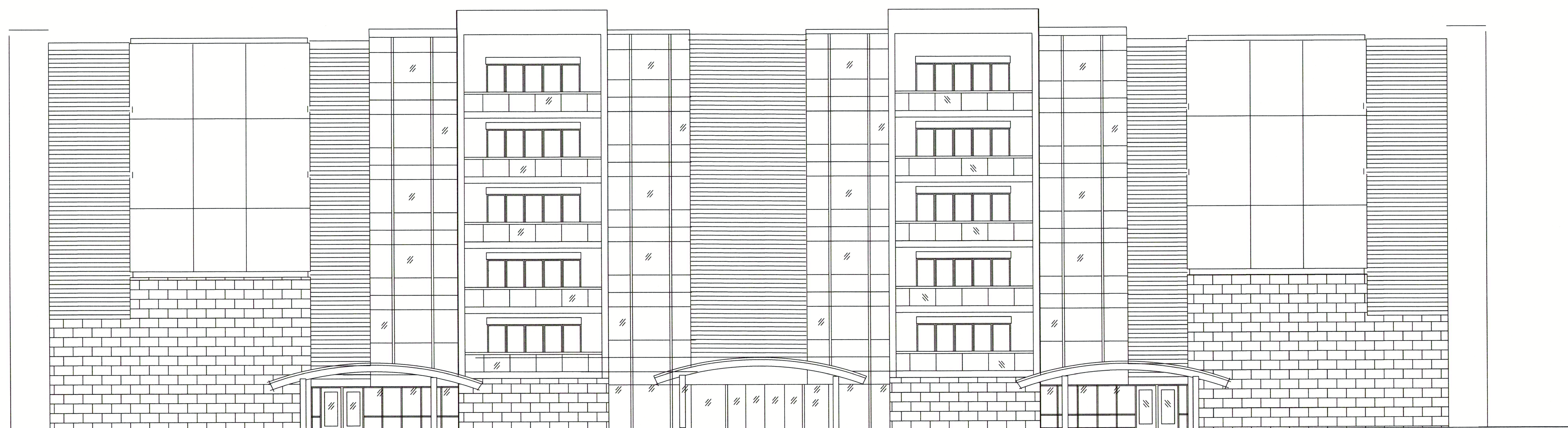
ELEVATION E MIXED BRICK AND EIFS AND HARDIE CEMENT FIBER BOARD
