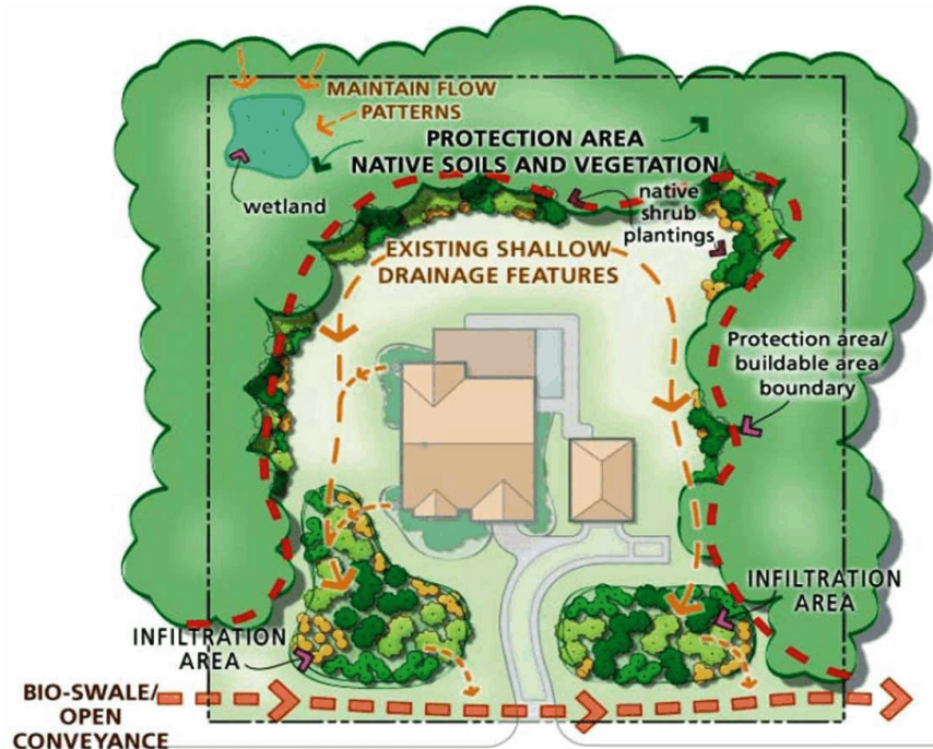
Figure 4-4. On Lot Treatment for Effective Stormwater Management (from Low Impact Development-Technical Guidance Document for Puget Sound, January 2005).
