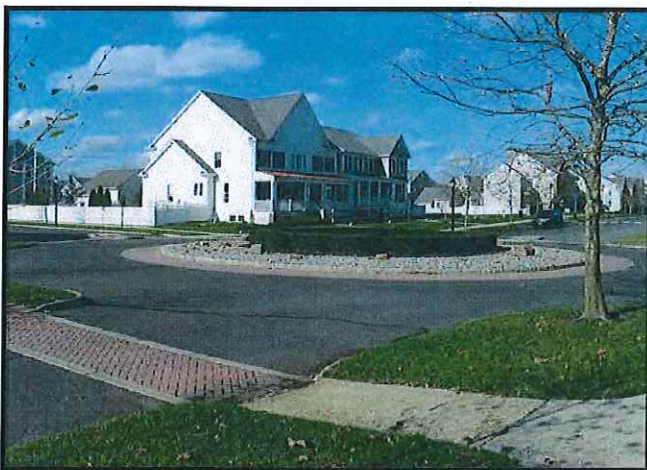
A decorative crosswalk contrasts with the cartway surface in order to promote visibility, and promote pedestrian circulation.
