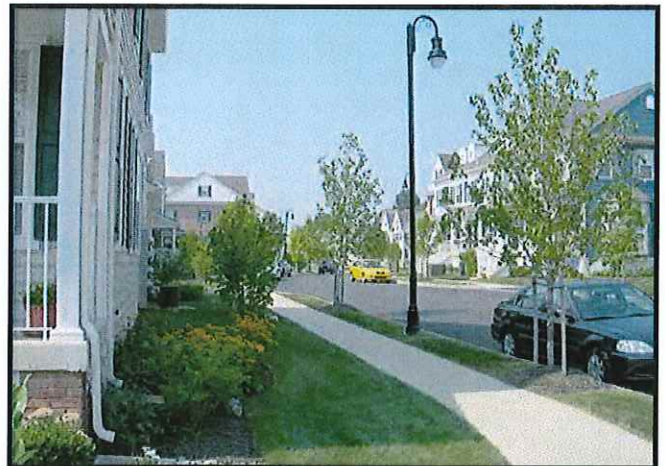
Accessway with on-street parking that is bordered with a sidewalk, grass strip, street trees and streetlights.
