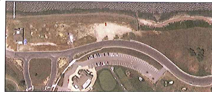
Aerial showing road realignment, sidewalks, and location of the installed gabion system. Source: GoogleEarth.
